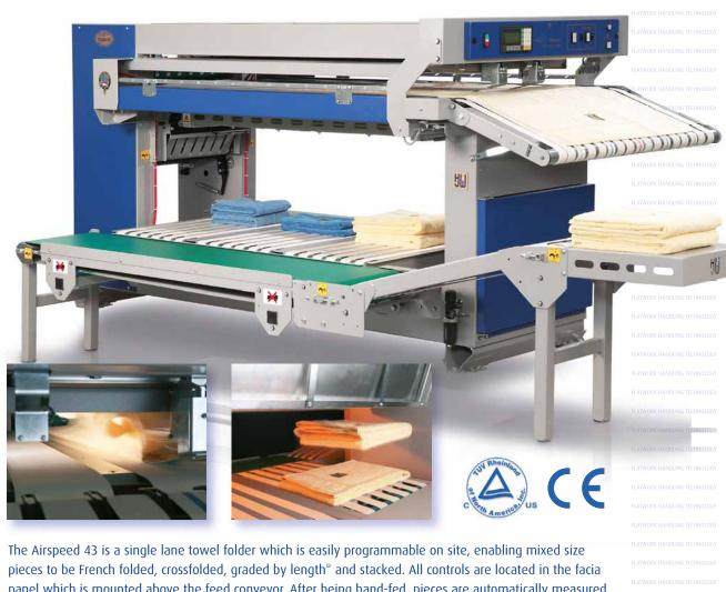
panel which is mounted above the feed conveyor. After being hand-fed, pieces are automatically measured for width and the machine adjusts to perform the perfect French fold. The piece is then conveyed to the crossfold section at which time Autograding\* takes place and up to two crossfolds added.
